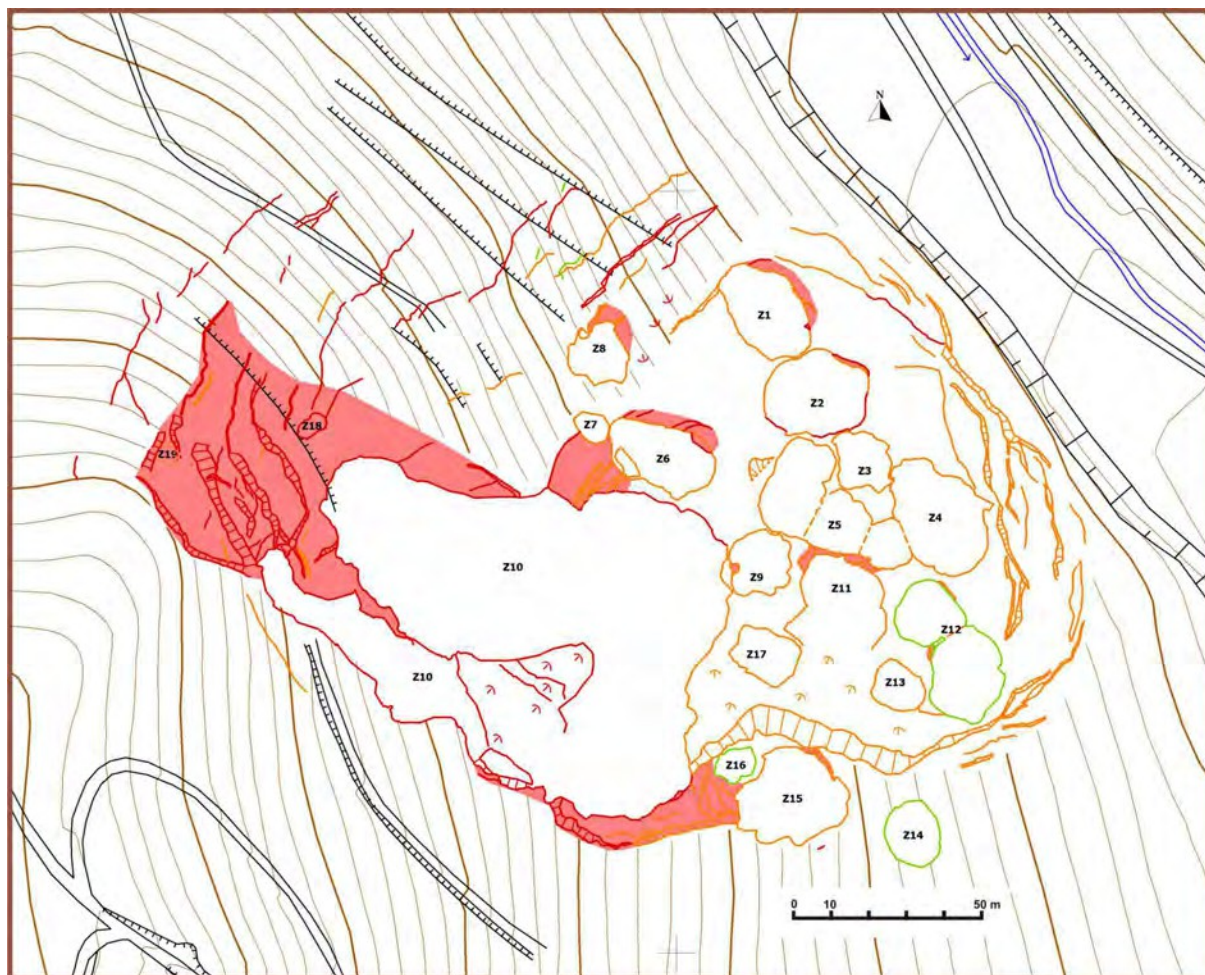
Fig. 30: Forecast expansion of landslides at the Kobeliarovo deposit marked with red areas (topographic base Ščuka et al., 1982).
