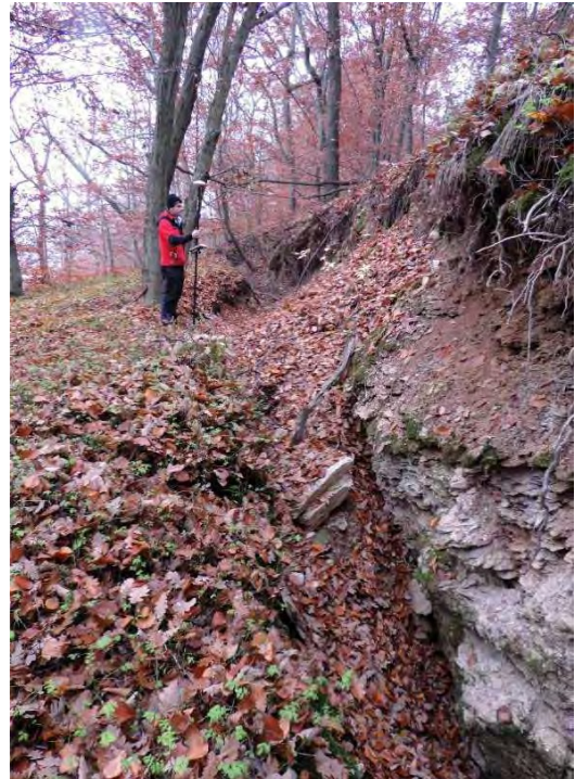
Fig. 10: Detachment surface of a significant tensile-subsidence fracture in the western part of the collapse area.
