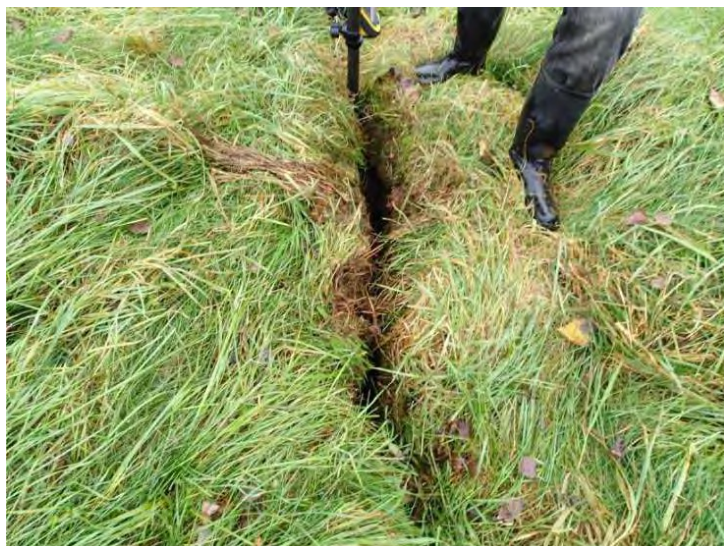
Fig. 18: Open tensile crack on the eastern edge of the collapse zone.
